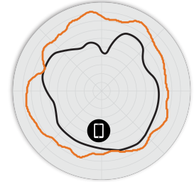
Figure 7. R770 6GHz Elevation Antenna Patterns
